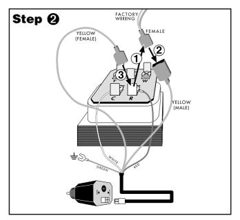
① Unplug the factory-wired quick connect from terminal **R** and ② plug into YELLOW wire with *male* connector. ③ Plug YELLOW wire with *female* connector into terminal **R**.
