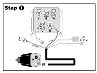
Connect the WHITE wire to **C** and the RED wire to **R** using the screw terminals on the control center. Connect the GREEN wire to any suitable, unpainted ground screw. **Note:** for operation of the control, the green wire must be connected to a ground source electrically common with boiler ground.
