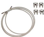
Safety Cable Kits are used as a secondary attachment on non-safety wheels to reduce the potential falling hazard of a falling valve hand wheel. The cable is fastened to the yoke of the chain guide and attaches to a nearby pipe or other secure object. Included in the kit is 7x19 stainless steel wire with 4 stainless steel clamps.
